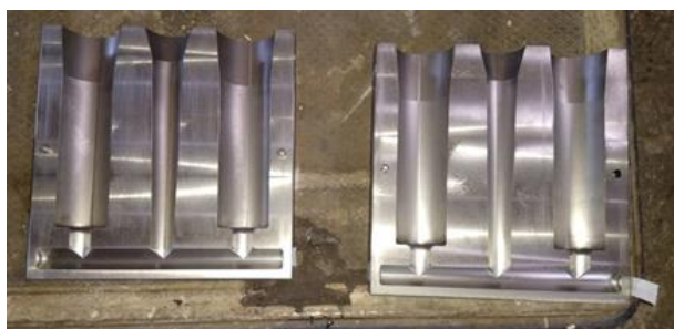
Fig. 1. Permanent mold used for casting the iron aluminide alloys investigated in this study
