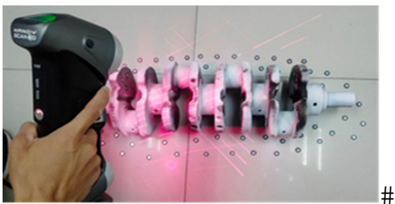
Fig. 7. The new crankshaft was created to artefact a 3D model by a 3D laser scanner
