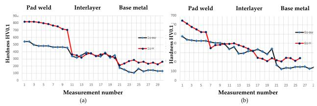
**Fig. 5.** Hardness HV0,1 distribution of pad weld, interlayer and substrate in cross-section and after impact hardening: a) samples: 1s-aw & 1s-H); (b) samples: 6s-aw and 6s-H
