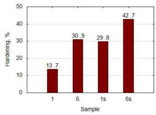
**Fig. 6.** Changes in sample hardness due to impact hardening, samples 1 and 6 – without interlayer, samples 1s and 6s – with interlayer
