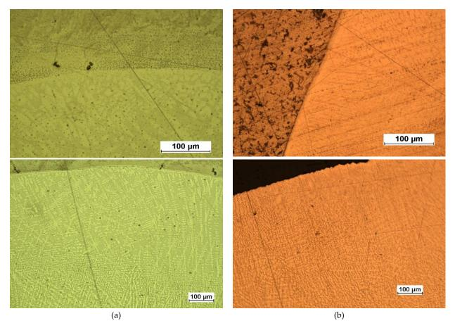
**Fig. 3.** Microstructure of stellite pad welds: (a) 1s-aw: 308LSi interlayer + EL-Co 1 pad weld; (b) 6-aw: S235JR substrate + EL-Co 6 pad weld
