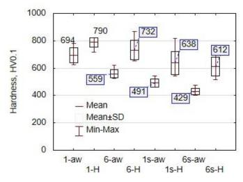
Fig. 4. Hardness of stellite coatings as-welded (aw) and after impact hardening (H)
