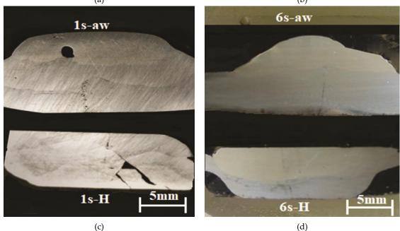
**Fig. 2.** View of as-welded (aw) and impact hardened (H) samples in cross-section: a) sample 1-aw & 1-H (cladded with Stellite 1 without interlayer); (b) sample 6-aw & 6-H (cladded with Stellite 6 without interlayer); (c) sample 1s-aw & 1s-H (cladded with Stellite 1 with interlayer); (d) sample 6s-aw & 6s-H (cladded with Stellite 6 with interlayer)
