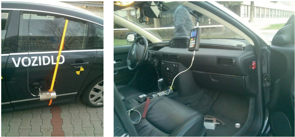
Fig. 5. Corrsys Datron Microstar measurement system mounted on the test vehicle
