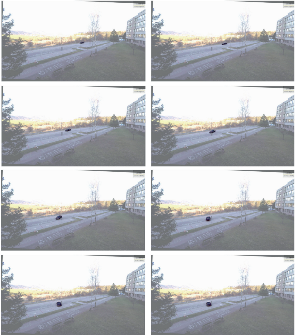
Fig. 9. Result of the vehicle movement reconstruction using VKM method - frames exported from composite video file in time step 0,5 s (test run A6)
