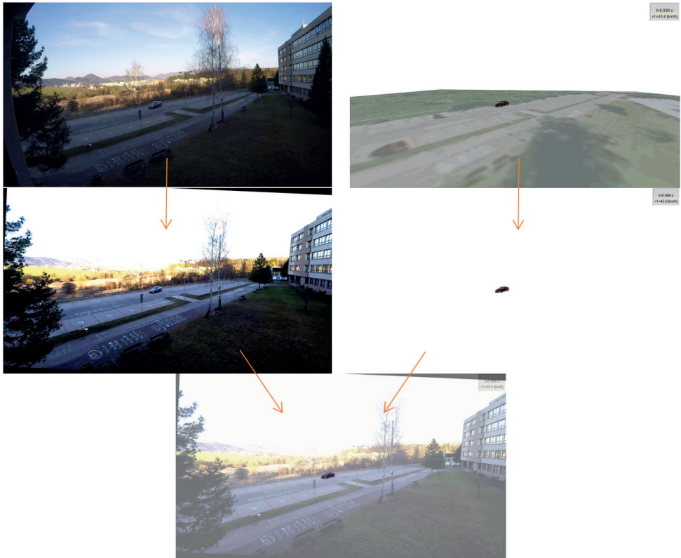
Fig. 8. Creation of composite video file shown on one frame: upper left – source (distorted) video, upper right – animation of simulation in PC-Crash (topography model depicted), middle left – undistorted and rotated video, middle right – animation of simulation in PC-Crash (topography model not showed), lower – composite video file
