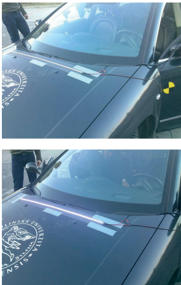
Fig. 6. View at synchronization LED strip
