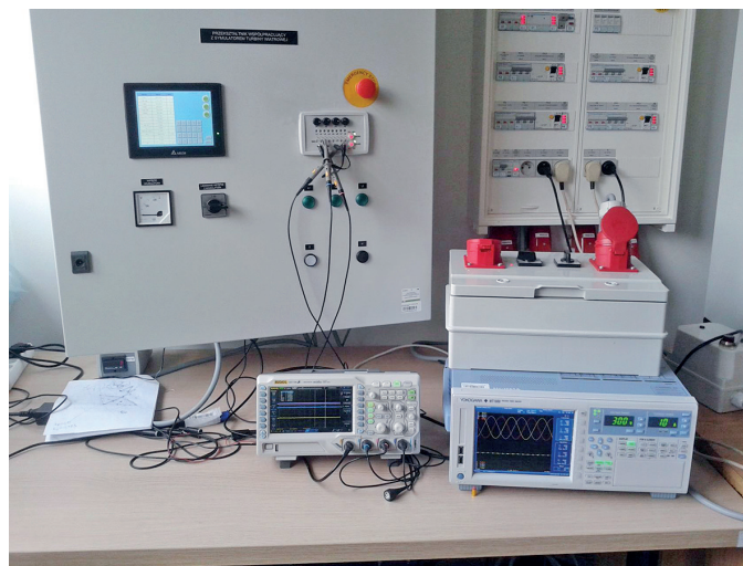
Fig. 8. Experimental setup of three-level AC-DC converter
