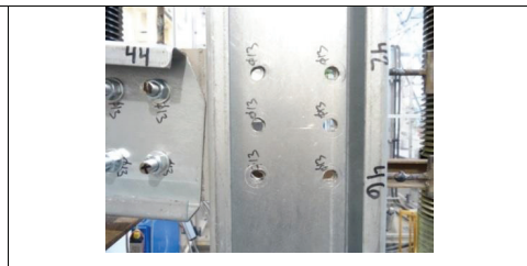
Fig. 11. Failure mode of specimen M12C15025I8
