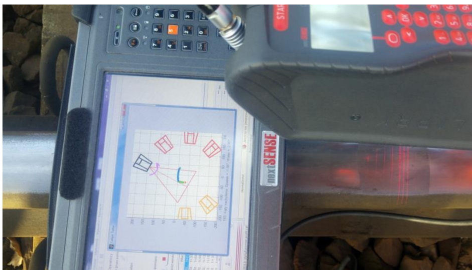
Fig. 2. View of the measurement of the head profile and rails welds after thermite welding
