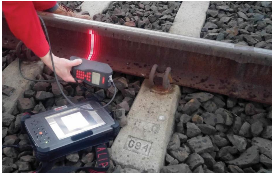
Fig. 3 View of the measurement with the Calipri laser device of the rail head profile 600 mm in front of the contactless joint of thermite-welded rails, the laser module in one of the seven measuring positions – auxiliary, side based
