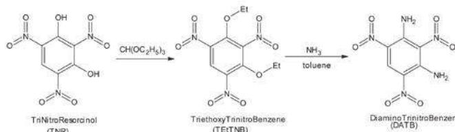
Fig. 2. Scheme showing synthesis of DATB from trinitroresorcinol
