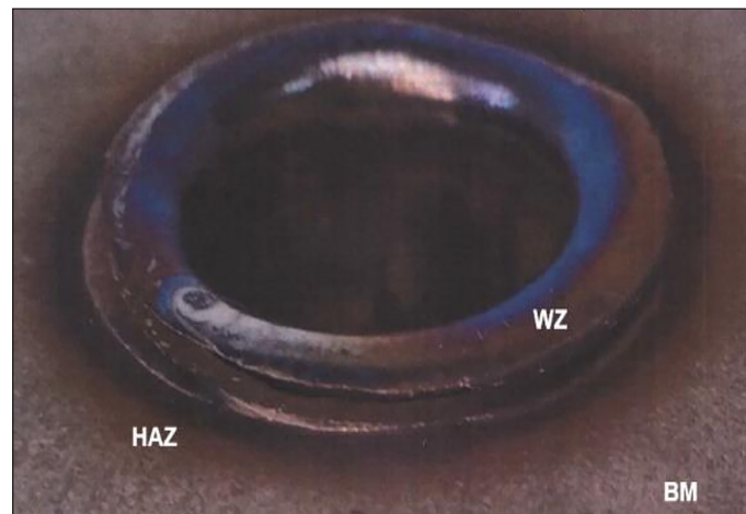
Figure 5. Places of measurement of the ferrite content in individual zones (BM – base material, HAZ – heat-affected zone, WZ – welding zone)
