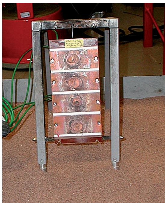
Figure 4. Copper-coated K-type thermometer for temperature measurements.
