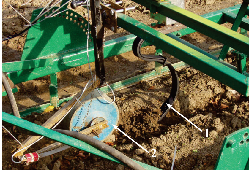
Figure 3. View of cultivator tine (1) and sensor wheel (2) mounted in test stand
