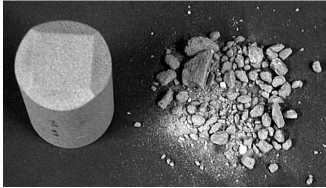
Figure 7. Ceramic projectile (strength: 80 N/mm 2 ) with front face in accordance with Standard No. EN 12415:2003 [4] before impact (left) and after impact (right), projectile energy: 9303 J.
