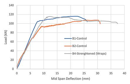
Figure 11. Load-displacement relationship of B4
