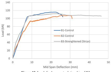
Figure 10. Load-displacement relationship of B3
