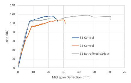
Figure 12. Load-displacement relationship of B5
