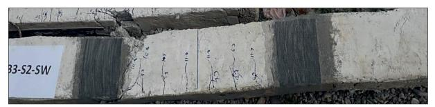
Figure 7. Final crack pattern of specimen B4 (strengthened with CFRP wraps)
