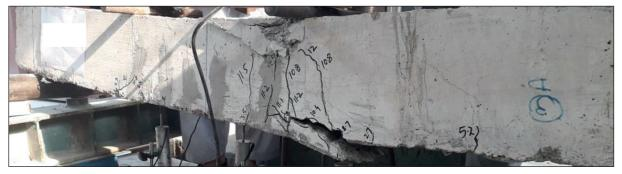
Figure 8. Final failure pattern of specimen B5 (retrofitted with CFRP strips)
