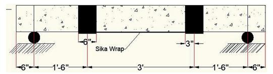
Figure 3. Side view of beams retrofitted by CFRP wraps
