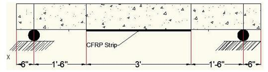
Figure 2. Side view of beams retrofitted by CFRP strips
