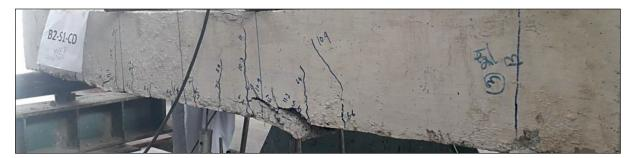
Figure 6. Final crack pattern of specimen B3 (strengthened with CFRP strips)
