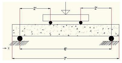
Figure 4. Schematic of test setup
