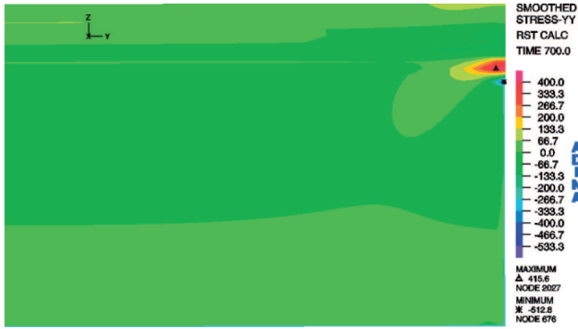
Fig. 10. Radial residual stress bands determined in a fragment of the coating/substrate system (Ti coating thickness 0.145 mm)
