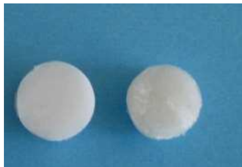
FIG. 1. Scaffolds made from the blend of Coll and SF.
