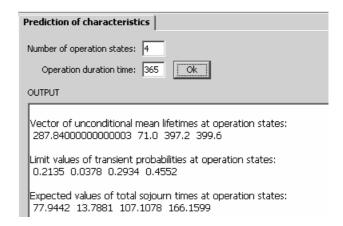
In above window there are given the unconditional mean sojourn times, the limit values of the exemplary system operation process transient probabilities at the particular operation states and the expected values of the total sojourn times  $\hat{\theta}_b$ , b=1,2,3,4, of the system operation process at the particular operation states  $z_b$ , b=1,2,3,4, during the fixed operation time  $\theta=1$  year = 365 days.
