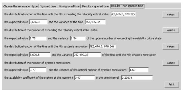
Integrated software tools supporting decision making on identification, prediction and optimization of complex technical systems operation, reliability and safety. Part 3 Integrated software tools application – Exemplary system operation and reliability characteristics prediction
