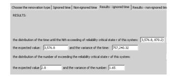
Each characteristic can be presented in the table of values for fixed parameter *t*. For example, the table of distribution values of the time until the *Nth* exceeding the reliability critical state and the table of distribution values of the number exceeding the reliability critical state are shown below.
