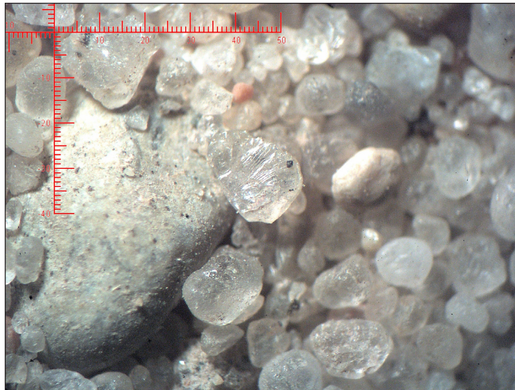
Figure 2. Natural sand, 25x magnification
