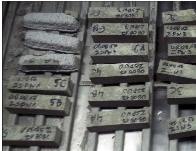
Figure 13. The samples after 100 freeze/thaw cycles. Clearly visible total destruction of the R0 samples
