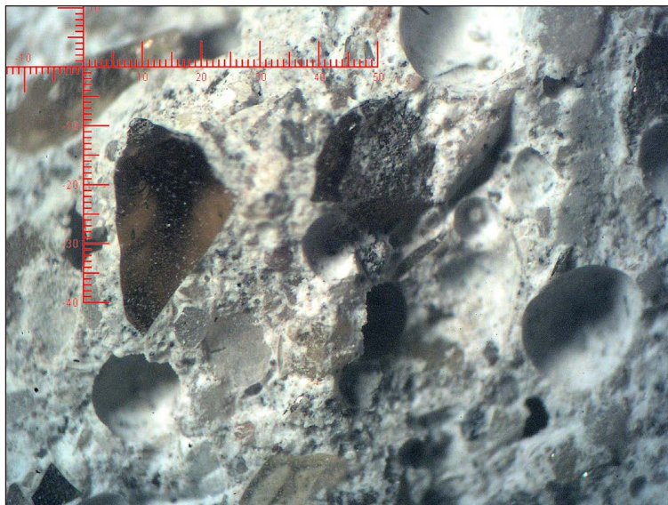
Figure 10. RWG3 mortar, 25x magnification
