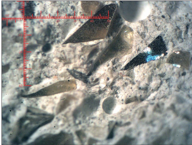
Figure 9. WG3 mortar, 25x magnification
