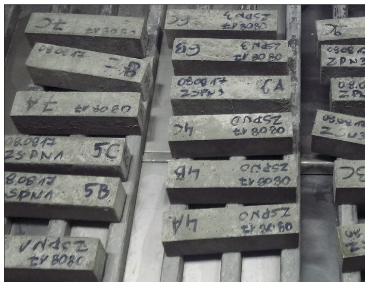
Figure 12. The samples after 25 freeze/thaw cycles
