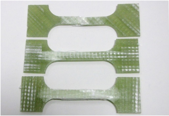
Fig. 10. Specimens of the composite (10 layers of reinforcement) after tensile test, taken from 45°, 0° and 90° direction, respectively
