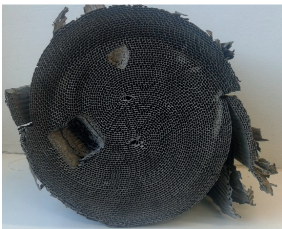
Fig 1. Metal Substrate Converter with corrugated FeCrAl foils, applied in experiment
