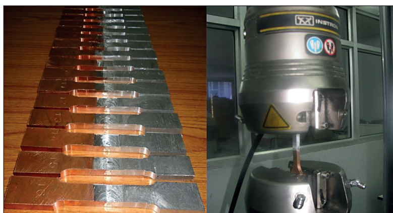
Figure 5. Tensile test specimen ASTM E-8 standards
