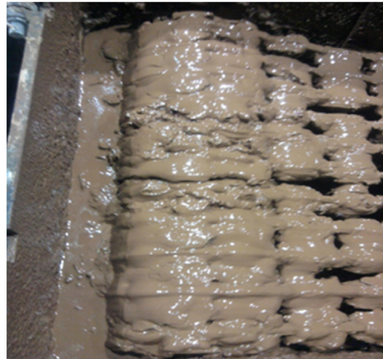
Fig. 5. A view of the test rig for wear tests filled with the abrasive mixture composed of quartz sand and water – at the initial stage of the tribocorrosive wear tests
