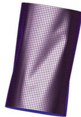
Fig. 11. An incorrect form of deformation obtained in case of too many elements
