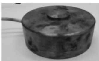
Fig. 4. Strain gauge measuring force of cutting
