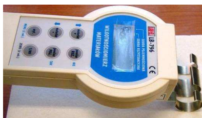
Fig. 1. Frequency Domain (capacitance) moisture meter (LAB-EL, Poland)
