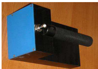
Fig. 2. Surface Time Domain Reflectometry probe (Lublin University of Technology)
