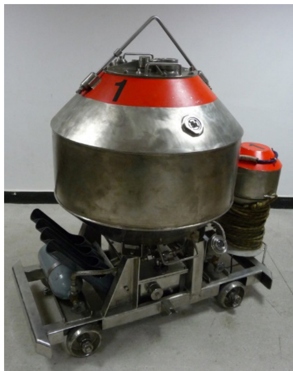
Figure 4 Station no 2 – MMDP with the trolley and equipment compartment
