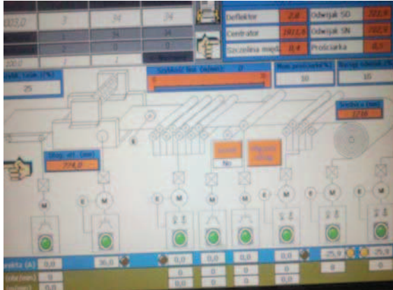
Fig.1. Screen of the system which controls the rollers power enabling the removal of sheet waviness
