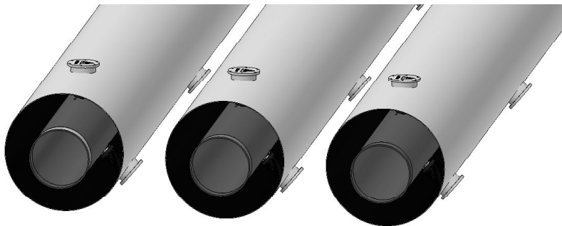
Fig. 1. Three-phase high-current busduct with isolated phases [11]
