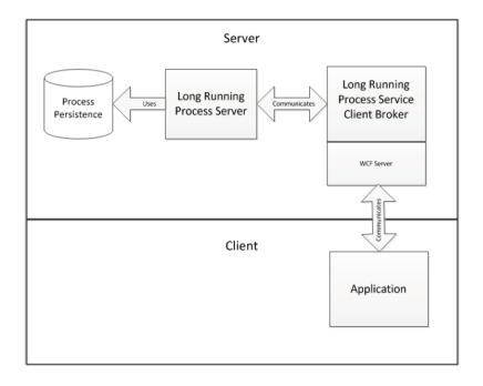
Figure 4. Architecture of the Long Running Process Server framework. Source: own design.
