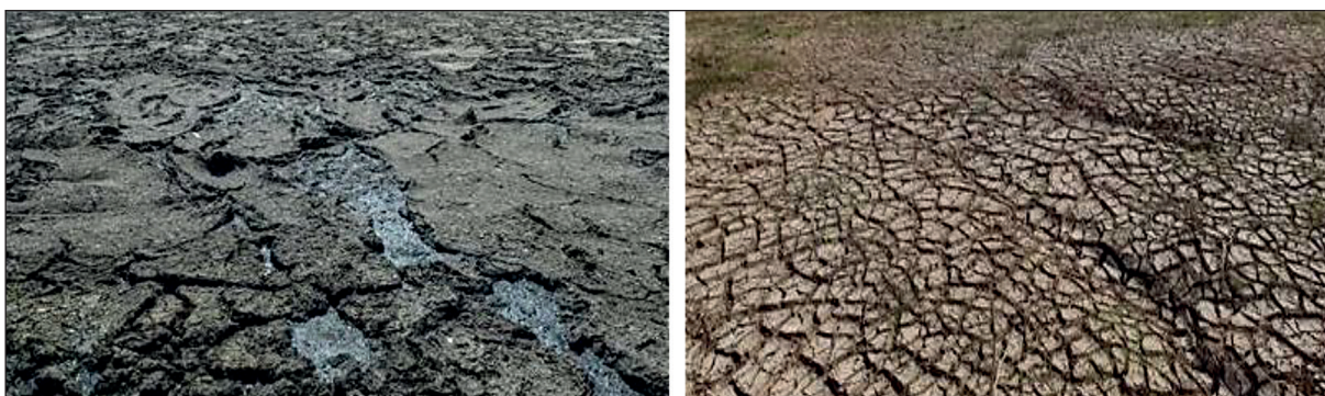
Fig. 2. Silts on the silt maps of the treatment facilities at Zhezkent; a) fresh sludge (no more than 1 week), b) naturally dried sludge (more than 1 month)
