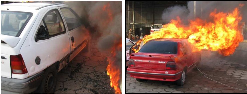
Fig. 1. Impact of the wind on the flame direction and the thermal impact of the burning car on the nearby car.
