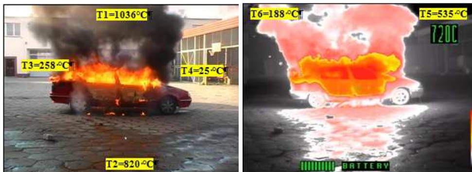
Fig. 2. A photograph and thermogram of car no. 1 in the phase of full fire development.
