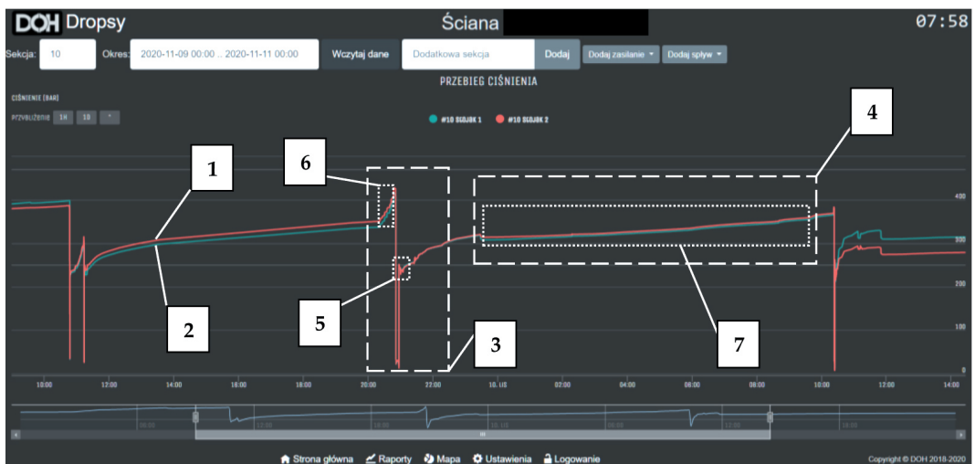
Fig. 11. The workflow of a powered roof support section: 1 – left leg, 2 – right leg, 3 – a time associated with the withdrawal, rearrangement and spragging, 4 – monitoring of section spreading in the longwall, 5 – initial support, 6 – nominal bearing capacity, 7 – working bearing capacity
