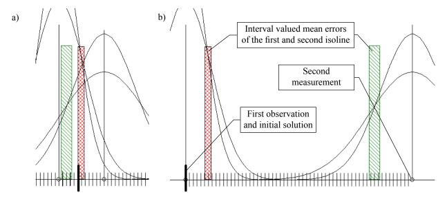
Figure 2. Two cases related to two pairs of observations made for two objects situated at opposite directions. Vertical rectangles refer to interval valued the standard deviations with respect to the measurements
