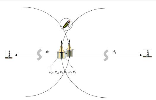
Figure 1. Graphical interpretation of two imprecise measurements, distorted with random and systematic errors, taken for objects at opposite directions
