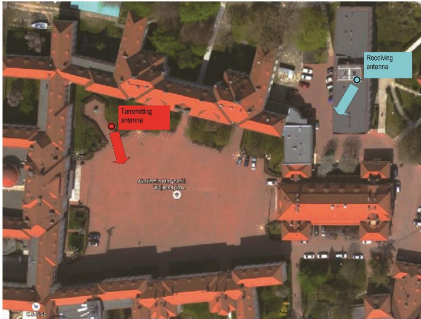
Fig. 6. The location of the antennas; transmitting and receiving, absence of direct reception
