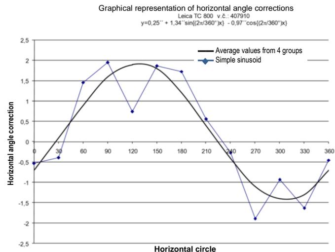
Fig. 7. Calibration curve and the approximating cyclic function
