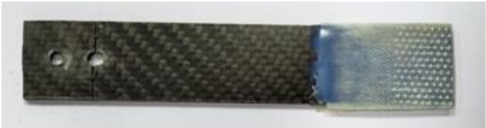
Fig. 7. Damage to the composite with a parallel orientation
