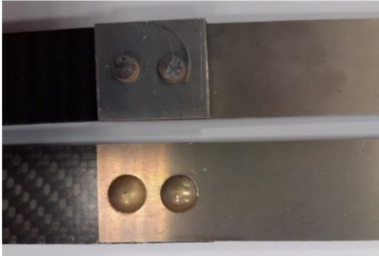
Fig. 4. View from two sides of a single-lap sample joined with solid rivets with the use of a spacer
