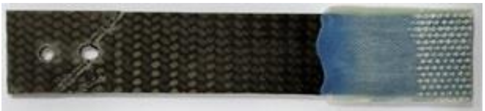
Fig. 8. Damage to the composite cut at an angle of 45°
