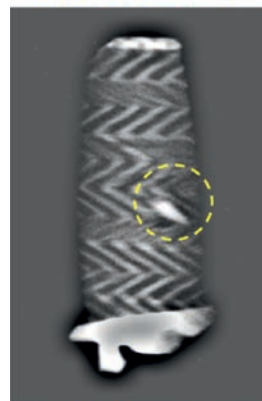
420 kV, 10 mA, 5 min, slit width: 0.9 mm (high-pass filtered)
