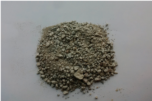
Fig. 1. Crushed concrete sample as used in testing
