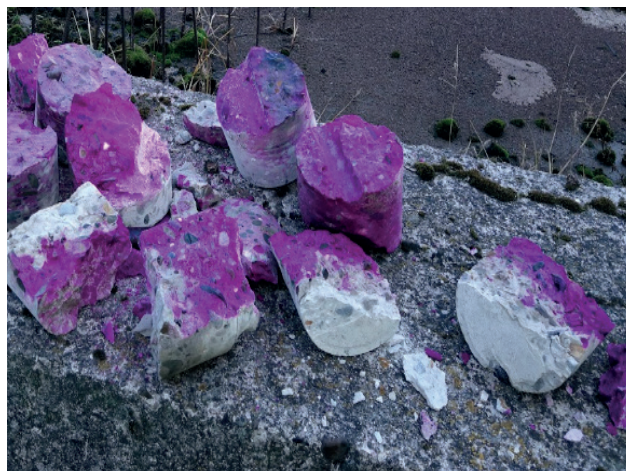
Fig. 6. Concrete carbonation tests
