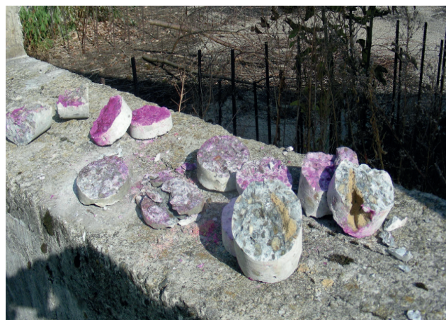
Fig. 4. Delaminated (impacts on concrete) samples. Right: a sample with poorly mixed concrete components – visible aggregate (sand) inside
