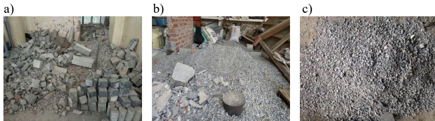
Fig. 2. CCA used in the study; a) before crushing, b) during crushing, and c) material used in the present study after crushing
