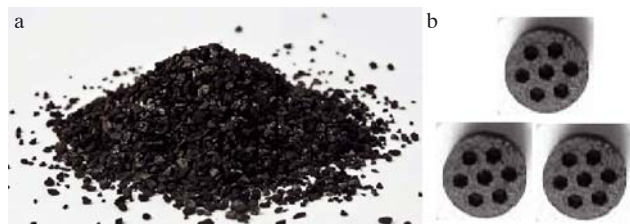
Figure 1. Carbonaceous materials a) granular activated carbon, b) activated carbon monoliths
