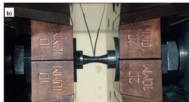
Fig. 2. Specially designed test sample (a) and the sample placed in simulator handles (b)
