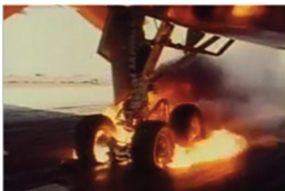
Figure 11. Burning brake in RTO test. RTO, rejected takeoff.
