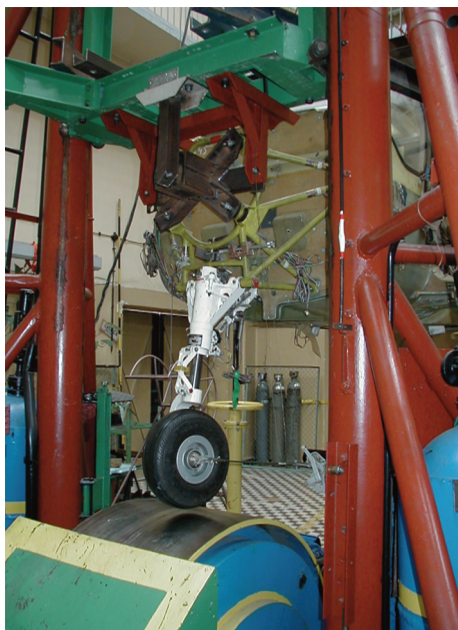
Figure 8. M3T/6T test stand – example aircraft LG test. Source: Landing Gear Laboratory, Ł-ILot.
