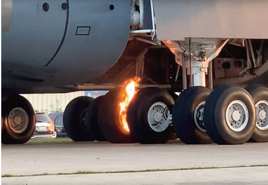
Figure 3. Burning aircraft brake. Source: The Aviation Geek Club https://theaviationgeekclub.com/watch-this-video-featuring-a-c-5m-super-galaxy-experiencing-brake-fire-at-oshkosh-airventure-2019/
