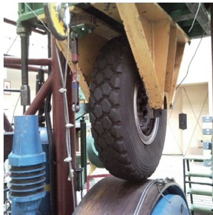
Figure 7. M3T/6T test stand – example of an armored full-scale brake test.
