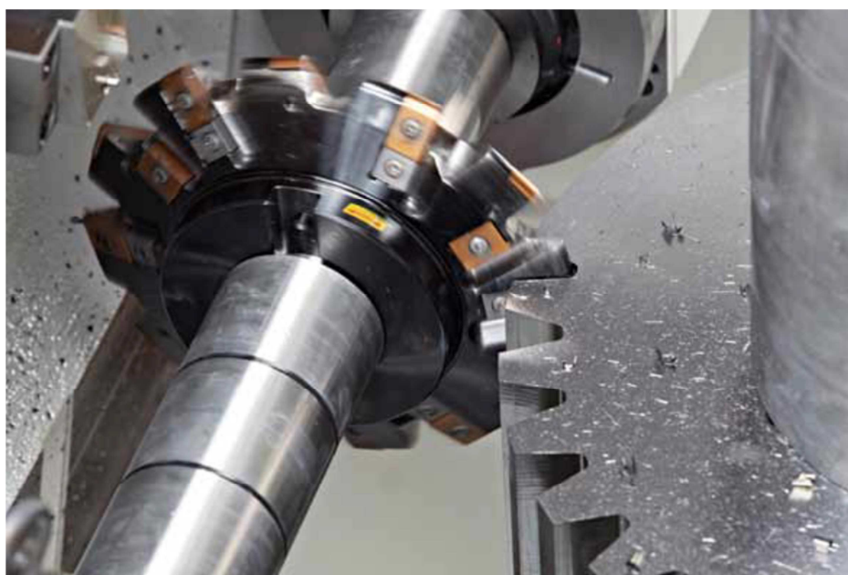
Fig. 5. Rough gear cutting with Coromill 170 [13]
