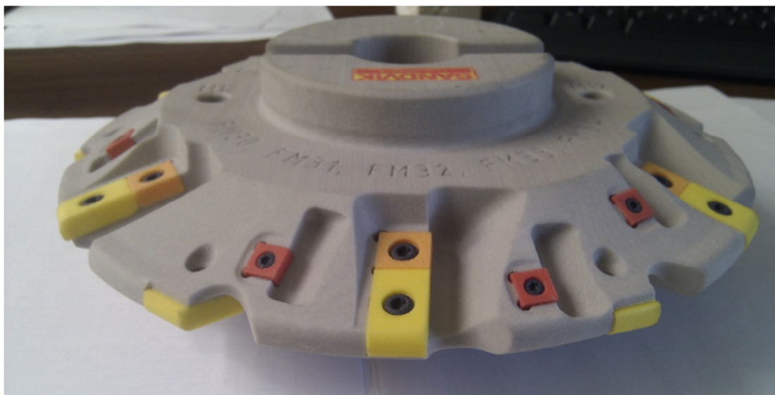
Fig. 4. Custom model of tool obtained with 3D printing technics [13]
