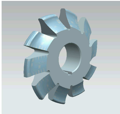
Fig. 1. 3D CAD model of uniform tool for gear milling [own design]
