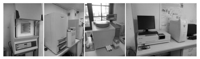
Figure 2. The lab equipment used in presented researches (from the left: muffle furnace; atomic absorption spectrometer – AAS - dedicated to the determination of carbon, hydrogen, nitrogen and sulphur content in solid materials; calorimeter bomb; AAS dedicated to the determination of mercury content in solid materials; ion chromatograph).
