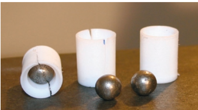
Fig. 3. Steel spherical projectiles with a diameter of 8 mm and Teflon sabots
