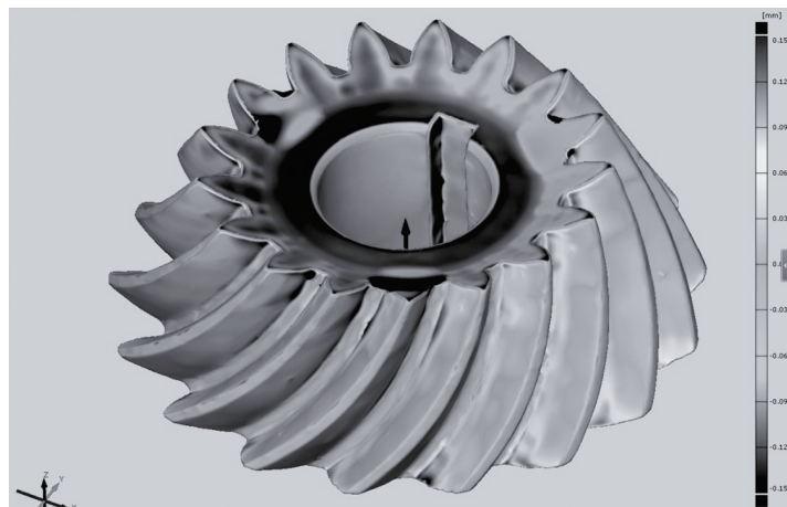
Fig. 6. deviations map obtained for the model made by PolyJet method
