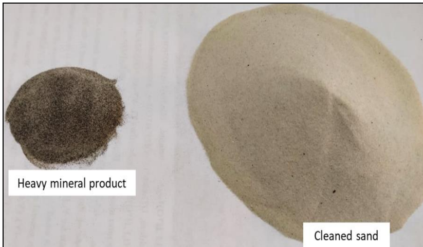
Fig. 17. Photograph showing shaking table separation products for El-Harra sand
