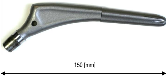
Fig. 1. General view of the fractured stainless steel stem
