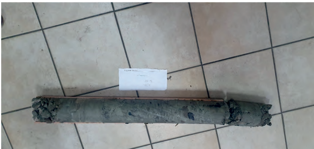
Fig. 3 The undisturbed soil samples from the internal dump of the KWB Konin mine
