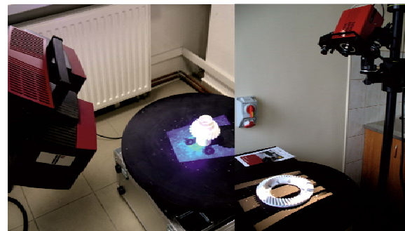
Fig. 3. Measuring of bevel gears using 3D ATOS optical scanners- blue and white and light
